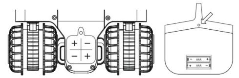
3. To power on the vehicle, switch vehicle button to "On' position, to power on the remote control, press the power button for approximately 1 second until the power LED lights up.
