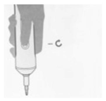
Press this button to rotate the screwdriver bit clockwise
