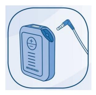
7. Press Power Button to turn unit on.(AC Charger must be disconnected from unit.)
