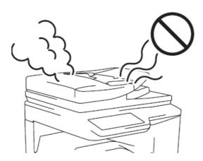
If a thunderstorm begins, switch off the main power and remove the power plug from the outlet to prevent electrical shock and fire due to lightning.
