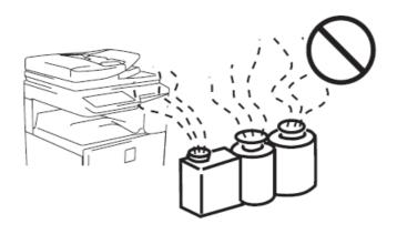
Opo not install the machine in a location with poor air circulation.
