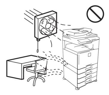
\* Install the machine so that people are not directly exposed to exhaust from the machine. If installed near a window, ensure that the machine is not exposed to direct sunlight.
