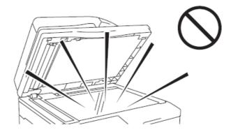
O Do not block the ventilation ports on the machine. Do not install the machine in a location that will block the ventilation ports.
