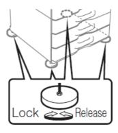
Rotate the adjusters in the locking direction until they are in firm contact with the floor.
