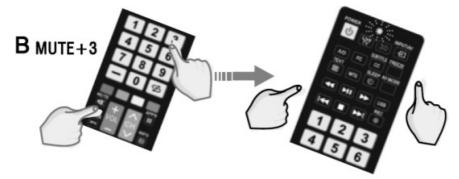
3. A remote control: Press and hold the MUTE and 1 buttons for more than 3 seconds. When the LED indicator lights up, release the buttons. When the LED on both remote control flash, the learning function is on. When the LED indicator on both remote controls flashes three times slowly then goes off, it means that learning has
