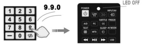
3. Input the numbers: 1, 2, 3. After pressing the 1 button, LED indicator starts to flash. The number of flashes is the code's first number. If the code number is 0, LED indicator will not flash.
