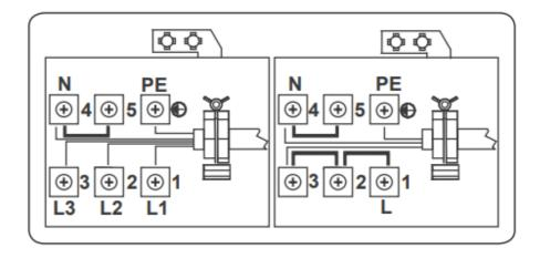
For the induction hob, the cable must be H05VV-F 3X4 mm<sup>2</sup> or 3x4mm<sup>2</sup> 60227 IEC 53 ••. You will find the connection diagram shown on the bottom of your appliance.
