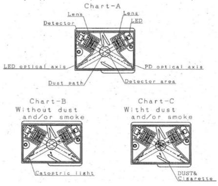
Light from the light emitter (Light Emitting Diode) is spotted with a lens and a slit as shown on the chart-A. Also for the light detector (Photodiode), a lens and a slit is positioned in front of it to cut disturbance light and to detect light reflection (when detecting dust) efficiently. Area where those two optical axis cross is detection area of the device.
