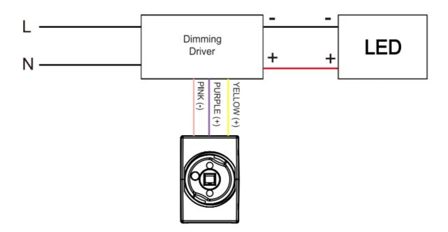
Wiring by AC/DC Adapter with dimming ballast or led driver.
