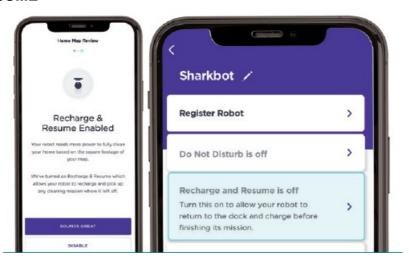
For optimum performance, your robot vacuum will return to the base, recharge, and can pick up where it left off. Turn on Recharge & Resume in your app™s Settings.
