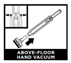
To detach the hand vacuum, slide the release tabs on both sides of the handle and lift it off the wand. Attach an accessory by sliding it into the nozzle. To remove the accessory, slide the release tabs on the handle. To reattach the hand vacuum, slide the nozzle over the wand on until it clicks into place.
