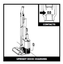
Charge the unit by placing it on the dock. Make sure the contacts on the wand are aligned with the contacts on the charging post.
