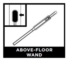
To detach the floor nozzle, step on the nozzle while pressing the release button at the bottom of the wand. Lift the wand to remove it. Reattach by sliding the wand over the nozzle neck until it clicks into place.
