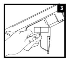
Wipe dust screen lightly with a dry cloth to remove dust and dirt.
