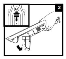
With the power off, slide the release button forward, and the dust cup will swing open. Tap the dust screen lightly to knock off dust and debris.
