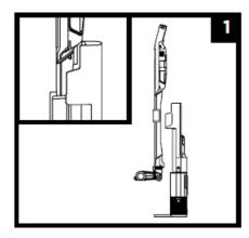
Place the vacuum on the dock in a downward motion. Once properly attached, the auto evacuation process will begin. The evacuation cycle will last for 10 seconds.
