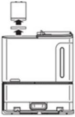
Allow the filters to dry for 24 hours before installing back into the base. After the filters have dried, place the felt filter, followed by the foam filter back into the base. We recommend cleaning the filter every two months and replacing it every 6-12 months. You can purchase a replacement filter from [sharkaccessories.com](http://sharkaccessories.com).
