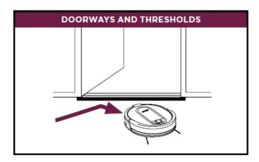
Your robot can easily climb over most thresholds but if one is higher than 7/8ths of an inch, block it off with a BotBoundary® strip.
