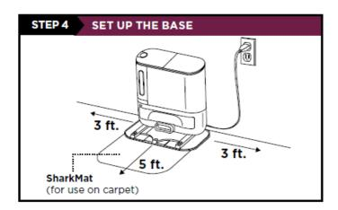
Find a permanent location for the base. Place it with its back against a wall, in an area with a good Wi-Fi signal. Remove any objects that are closer than 3 ft. from either side of the base, or closer than 5 ft. from the front. For best results, set up base on hard floor, or on the SharkMat.
