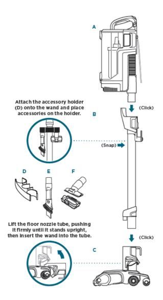
**NOTE**: For proper operation, ensure all parts are firmly CLICKED into place.
