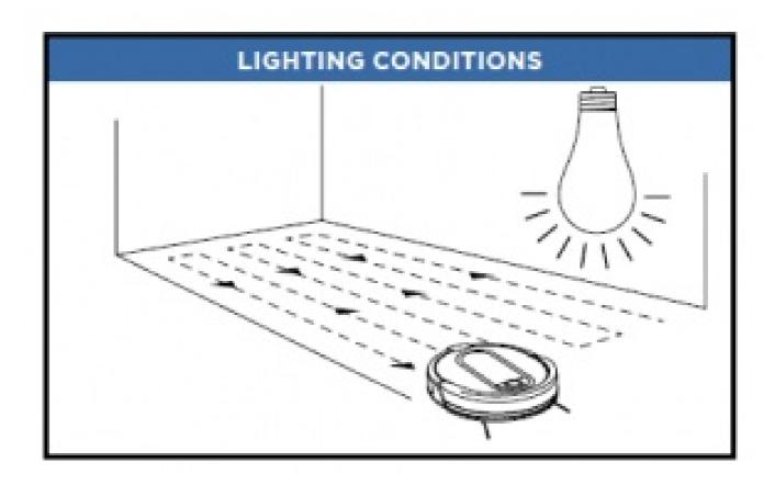
For best results, run your robot in well-lit conditions. If you run your robot at night, keep the lights on in the areas to be cleaned.
