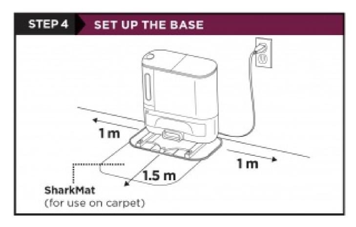
Find a permanent location for the base. Place it with its back against a wall, in an area with a good Wi-Fi signal. Remove any objects that are closer than 1 m from either side of the base, or closer than 1.5 m from the front. For best results, set up base on hard floor, or on the SharkMat.
