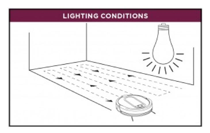
Your robot has a hard time navigating your home in the dark. Run your robot in well-lit conditions. If you run your robot at night, make sure to keep the lights on in the rooms to be cleaned.
