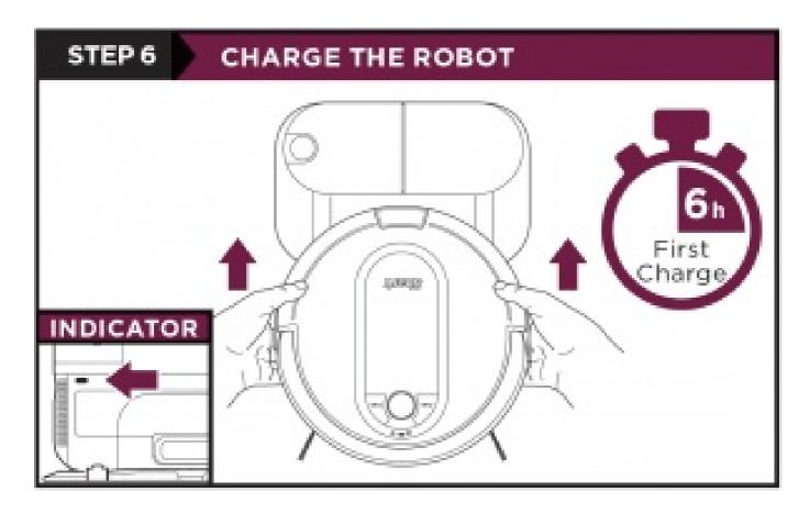
Place robot on base to charge for 6 hours. Power button must be in the (I) ON position and the robot must be aligned correctly, with its back side against the base. When charging begins, the robot will BEEP and the DOCK light will turn BLUE.
