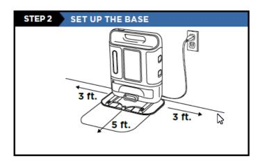
Find a permanent location for the base. Place it with its back against a wall, in an area with a good Wi-Fi signal. Remove any objects that are closer than 3 ft. from either side of the base, or closer than 5 ft. from the front. For best results, set up base on hard floor.
