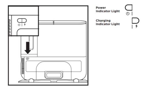
There are 2 indicator lights on the front of the base, the green power indicator light and the blue charging indicator light. When the base is plugged in and the power switch is turned on, the GREEN power light will illuminate. When the robot is charging on the base, the BLUE light will pulse. When charging is complete, the blue light will illuminate steadily.
