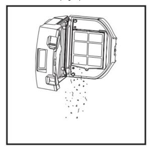
• Empty debris and dust into trash.
