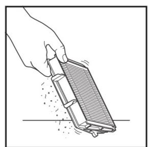
**IMPORTANT:** DO NOT use water to clean the robot filter.
