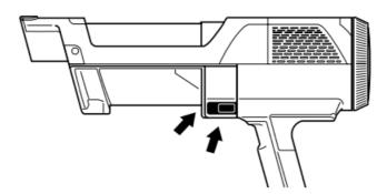
**IMPORTANT:** DO NOT use soap when cleaning the filters. Use water only. The vacuum will not have suction if the post-motor filter is not installed. Ensure that all filters are installed before using.
