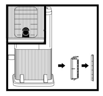
To access the hand vacuum filter, press the release buttons to remove the dust cup, then remove the filter from the housing.
