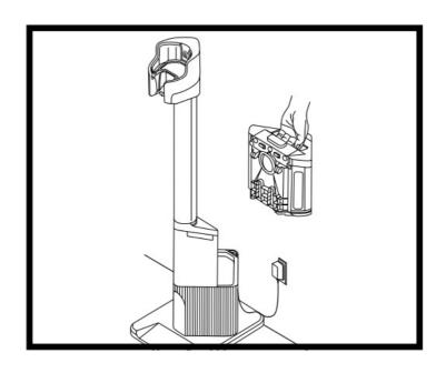
To remove the bin, press the release button and lift the bin out by the handle. To empty the bin, hold it over the trash and press the release button located on the top face of the bin. The bottom will open to release the debris.
