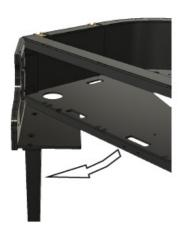
Loosely thread the sled hardware with the carriage anchor knobs, Do not fully tighten at this step.
