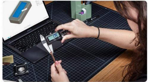
Use the Connected Caliper to send measurements to your computer or tablet running your favorite CAD tool or spreadsheet.
