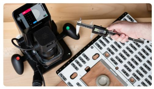
By pressing the yellow button, the Connected Caliper will send your measurement to Origin – automatically populating the dimension, from cut depth to part geometry.
