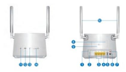
WPS Button LAN Port USB port Power Switch SIM Card Power LED LTE LED
