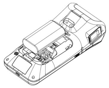
4. Put the battery door back. Press the ON/OFF key to power on.  $\,$
