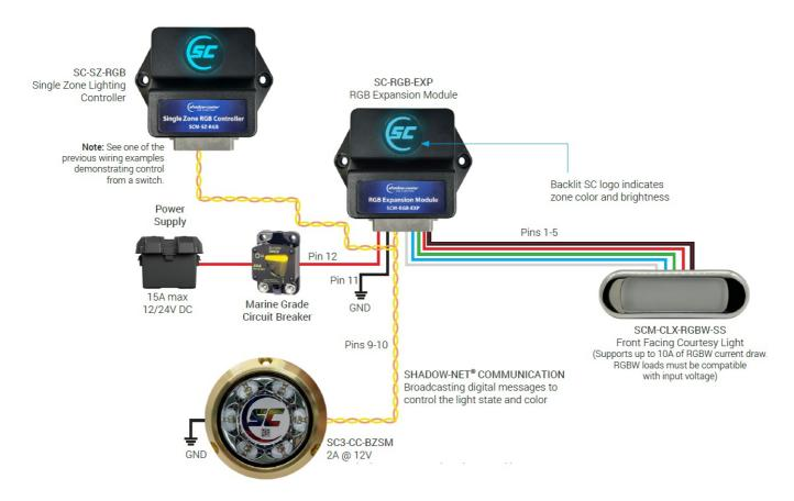
Note: Shadow-NET's current draw does not add to the 10A budget for the Single Zone controller
