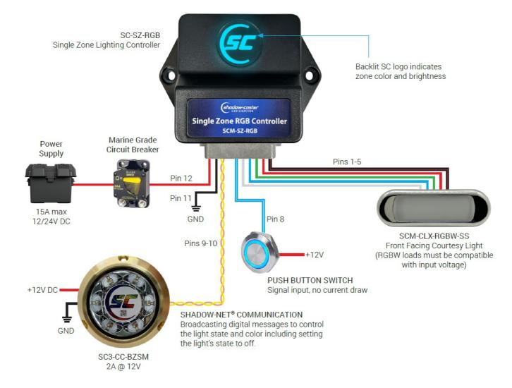
Note: Shadow-NET's current draw does not add to the 10A budget for the Single Zone Controller
