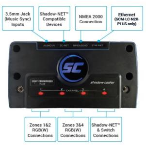
The Light Commander has four built in RGBW channels. By default these RGBW channels correspond to zones 1-4, identified in the device list as "LOCAL 1-4" (see Configure Devices screen shot on page 11). However, they are independent and can be assigned to any of the configured zones 1-6 supported by the controller. The Light Commander will support 15 amps on each of the 4 RGB(W) channels, for a total of 60 amps in the entire Light Commander.
