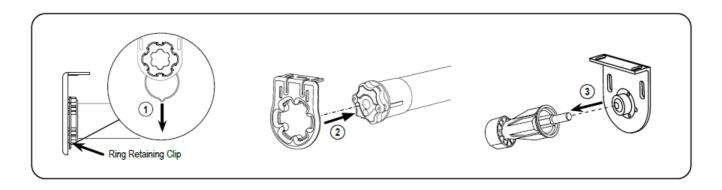
**Note:** Illustration shown under Open Roll without top treatment, same concept applies to Fascia & Pocket. First, raise the shade. Remove the ring retaining clip in place from the motor. Then, slide the roll towards the spring loaded pin end until the motor head are completely out of the motor head slots. Lastly, remove the spring loaded pin end from the Idler bracket.
