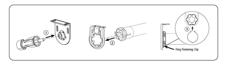
**Note**: Illustration shown under Open Roll without top treatment, same concept applies to Fascia & Pocket. Install the shade with the motor brackets (A and B) following the steps in the provided Roller Shades Installation Instructions.
