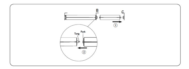
Note: Illustration shown under Open Roll without top treatment, same concept applies to Fascia & Pocket. Install the final bracket (C) level and aligned to the other brackets, following the steps in the provided Roller Shades Installation Instructions.
