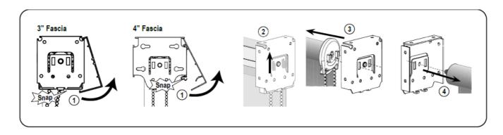
First, rotate upward to disengage the fascia. Then, gently pull up the control unit (Clutch, Motor or Spring) until the hooks touch the top part of the bracket slot. Pull the shade towards the spring loaded pin end until the hooks are complete out of the bracket slots. Finally, remove the spring loaded pin end from the idler bracket.
