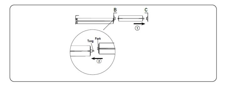
Note: Illustration shown under Open Roll without top treatment, same concept applies to Fascia & Pocket. Install the final bracket (C) level and aligned to the other brackets, following the steps in the provided Roller Shades Installation Instructions.
