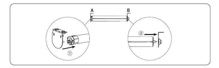
**Note:** Illustration shown under Open Roll without top treatment, same concept applies to Fascia & Pocket. Install the shade with the motor brackets (**A** and **B**) following the steps in the provided Roller Shades Installation Instructions.
