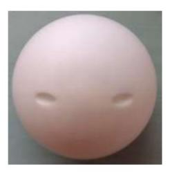
Movement Sensor Device is a device designed to measure parameters that detect possible movement in the grain and generates an alarm. The device consists of a board with an accelerometer that transmits data via LoRaWAN technology. The main purpose of the device is to obtain these acceleration values when the device moves. The whole device is shown in following figure:
