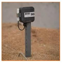
• The device covers an area of 8m of diameter and 350 Tons of grain:
