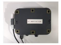
Then you can replace directly the 3 x AA batteries inside the case with standard AA commercial batteries. Screw again the case, assuring the correct assembly of all parts and check all the screws are properly tightened. Ensure the rubber seal is located in the plastic channel to prevent damage to it and to maintain the IP rating and protection.
