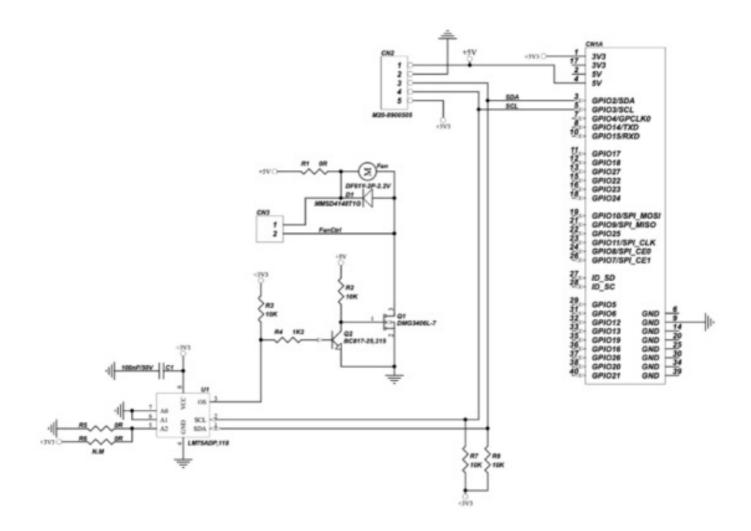
STRATO PI FAN CIRCUIT SCHEMATIC
