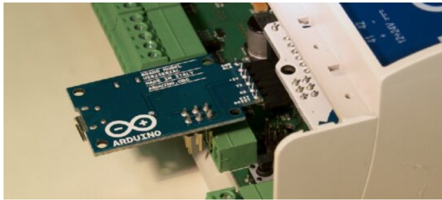
SERIAL ADAPTER CONNECTED TO THE ARDUINO BOARD
