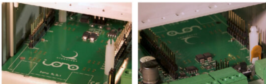
TURRETS INSTALLED ON THE IONO UNO BOARD
