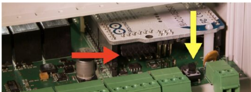
USB ADAPTER CONNECTOR AND RESET BUTTON
