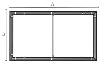
• Drill 4 holes in the wall at the desired height. The two holes horizontal distance should be 2/3 A, the vertical distance should be B minus 4 1/8" (105mm).
