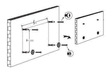
Hammer the expansion bolts into the 4 drilled holes, and drive 2 round head self-tapping screws into the upper expansion bolts, leaving about 1/4" (5mm) extended for hanging the screen on. Install the lower 2 magnet pieces using 2 flat self-tapping screws. Hang the screen on the upper brackets and attach the lower frame to the wall using the magnets.
