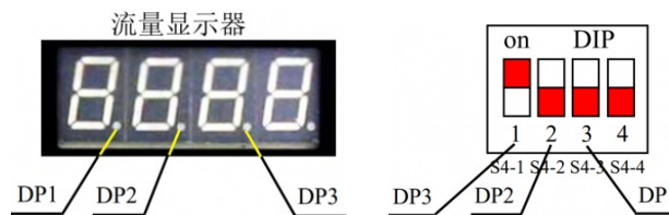
Figure 16. The Related Switches Positions Of Radix Point Modifying
