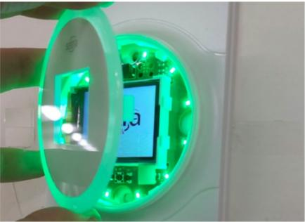
8. After configuration is completed align and engage the top two snaps. Then, align and install the front lens to the
