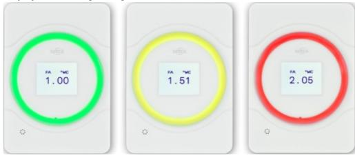
Setra Filter Alert features an LED light ring that changes color based on the pressure differential and the user defined thresholds. The light ring will glow green when the filter health is good, yellow when the filter needs changing soon but is still acceptable for use, and red if the filter needs to be replaced.
