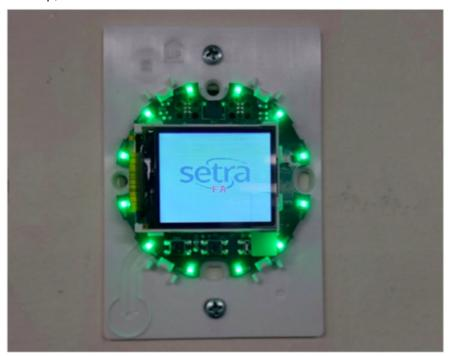
Setra Filter Alert contains a small air valve to allow for one-touch zeroing via the configuration menu.
