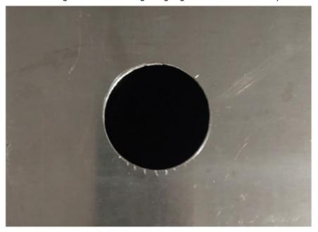
2. Install flush mount adaptor plate over clearance hole with four sheet metal screws (Customer provided). Ensure mounting holes for the base unit are aligned properly for orientation ordered (landscape or portrait).
