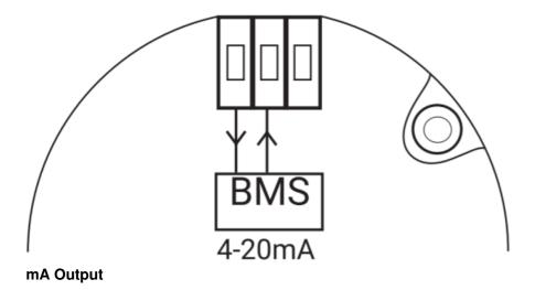
If using the Analog Output (AO) for voltage output, connect to the terminals as labeled on the left diagram above. If using the AO for mA output, connect to the terminals shown in the right diagram above. A 250 Ohm resistor is included for this output type in the event you need to convert to volts (1-5V). The AO generates a 0-5 VDC, 0-10 VDC, or 4-20 mA output signal, as configured.
