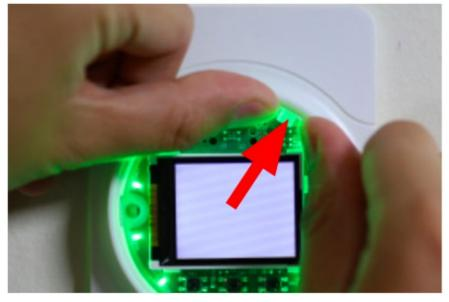
Once the faceplate has been removed, unscrew the unit from the wall or electrical box, and disconnect wires and pressure tubing.
