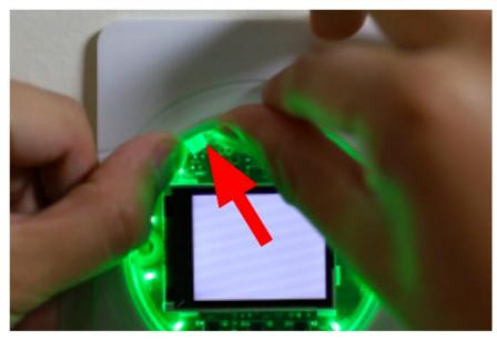
Next, locate the 4 snaps holding the faceplate to the unit. Carefully push on the inside lip of the faceplate near each snap to disengage each snap one at a time.
