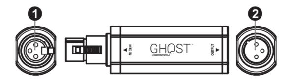
1. **INPUT:** use 3-pin XLR to connect SES-GHOST and passive ribbon microphone or dynamic microphone.
