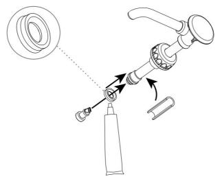
3. Install gaging collar onto side of head assembly piston.
