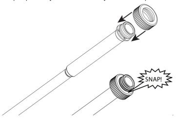
6. Install head assembly in cylinder. Apply small amount of food equipment lubricant inside top of cylinder and outside of seal. Slide locking collar down onto cylinder threading. Tighten firmly.
