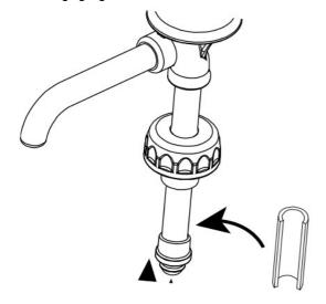
4. Insert spring into cylinder. For BP 1/2, add extension tube to bottom of cylinder to extend length.
