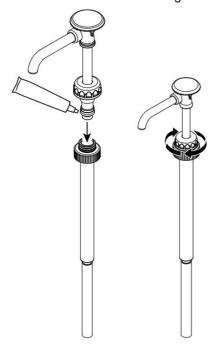
7. Insert and secure pump to product container. Tighten cap very firmly onto product container threading.
