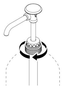
8. Prime pump by continuously pressing on the pump until prime is achieved.
