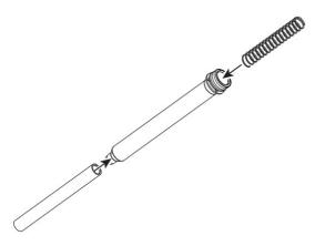
5. Snap cap onto cylinder. Press firmly to secure cap down over all threading on cylinder
