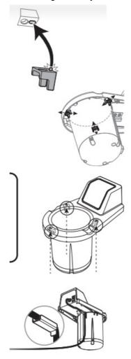
6. Insert green pan liner into the bottom of the pan. Fill 28 oz. of hot water up to the fill-line of the pan. Insert pan of water into a basin. Pour water into the pan only, never directly into the basin. Plug the cord into a power source. Press switch on the back of the unit to turn unit on. Press RESET to start the countdown timer.
