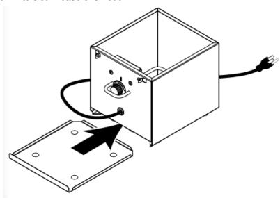
3. Insert dip container into shroud. Position #10 can(s) or stainless steel jar(s) between bumps at bottom.
