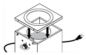
5. Install lid onto shroud. Align lid hinge holes onto pivot pins on shroud. Press lid hinges inward towards each other until pivot pins fit into hinge holes.
