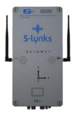
The S-lynks Gateways collect the data transmitted by the Nodes positioned on a structure.
