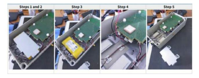
To connect a new battery pack, repeat the operation in the reverse order or consult "Connect the internal batteries of the Gateways".
