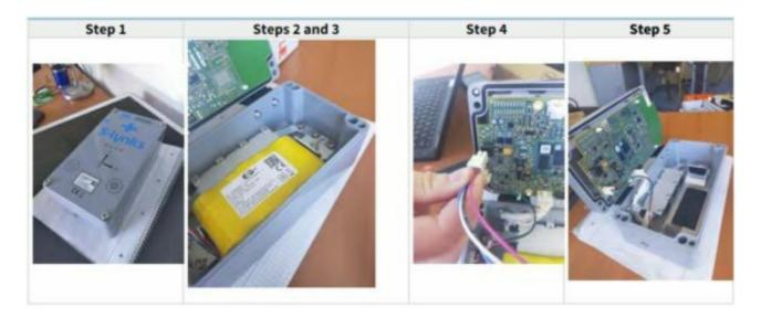
To connect a new battery pack, repeat the operation in the reverse order or consult "Connect the internal batteries of the Nodes".
