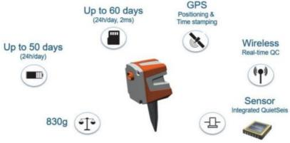
The AFU is the WiNG system's Analogue Field Unit (ref. 10042274). It is a single channel autonomous node including an external KCK2 connector for geophone. It includes communication capabilities to wirelessly deliver its QC status.
