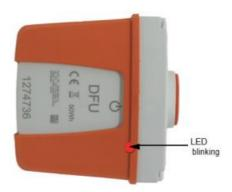
In case of problems detected during startup, the LED will blink 2 times per second. If a fault is detected, the geophones and their planting should be investigated.
