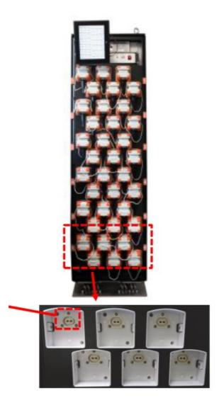
Connect field units to the Rack. The LED on the Field Unit will remain lit. See the WiNG Installation Manual, section fixing Field Units to Rack
