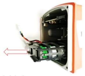
5. Put the new battery in the two shock absorbers.
