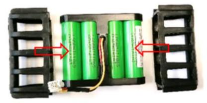
6. Place BATTERY PACK in place, take care of the orientation of both parts.
