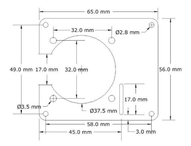
The Smart Fan has the same form factor with the Raspberry Pi HAT.
