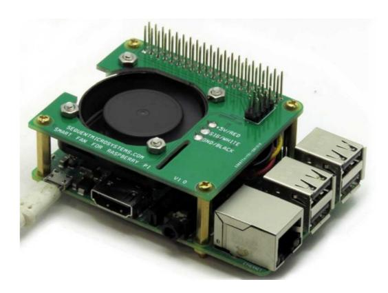
The Smart Fan is the most elegant, compact and inexpensive cooling solution for your Raspberry Pi. It has the form factor of the Raspberry Pi HAT. It receives commands from Raspberry Pi through the I2C interface. A step-up power supply converts the 5 Volts provided by Raspberry Pi to 12 Volts, ensuring precise speed control. Using pulse width modulation, it powers the fan just enough to maintain a constant temperature of the Raspberry Pi processor.
