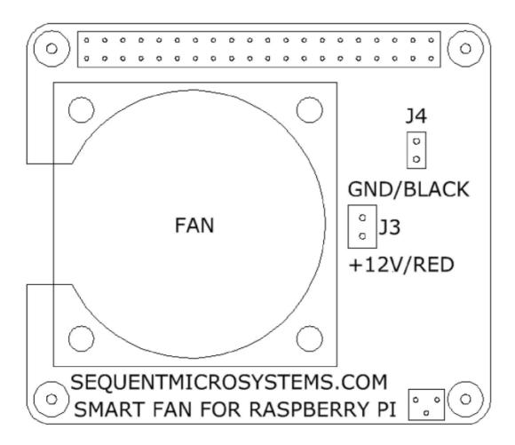
The Smart Fan comes with appropriate mounting hardware. All surface mount components are installed on the bottom. The fan is power from the Raspberry Pi GPIO connector and it draws less than 100mA. One or two fans can be installed on each Raspberry Pi. If the second fan is present, a jumper has to be installed on connector J4.
