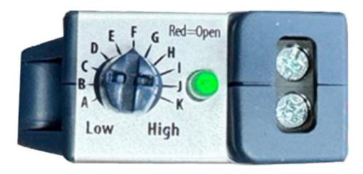
5. Note the position of the knob. For similar motors and applications, the same dial position can be applied to save calibration time.
