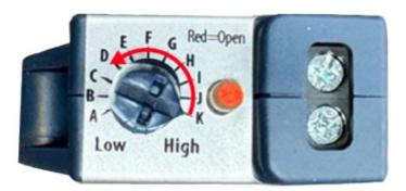
3. Once LED changes to green or relay closes, adjust dial up (CW) to nextlabeled position.
