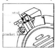
The sharpener is equipped with two grinding wheels, one is for sharpening the blade the other one is for repairing the edge. Press the button when sharpening the blade, rotate the blade, and press the end of the grinding shaft by hand, allowing the grinding stone to touch the blade. When sharpening the blade, you should press the end of the grinding shaft by hand to remove burrs from the blade being careful not to excessively grind the blade.
