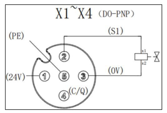
3. The IO-Link port is connected to the ULK-EIP-4A4BP6 substation. (When the IO-Link device is an input type, the 2 pins allow no wiring.
