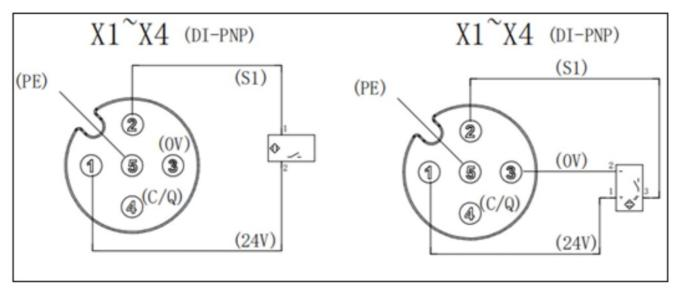
2. PNP type output signal, that is, the jack is connected to the actuator
