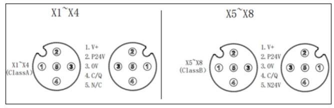
5.2.3 ULK-EIP-4A4BP6 IO Process Image Area Allocation 8-way IO-Link Interface (4 Class-A, 4 Class-B
