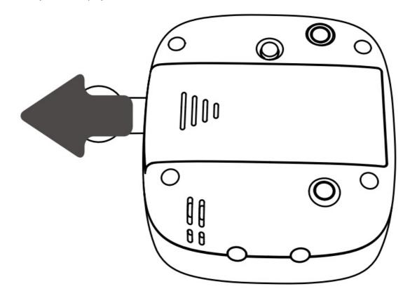
4. Long press the pair button on the back side of the product to switch between C/F.
