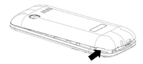
• Lift the battery with a LOUr nail or a flat tool on the phone's top part in the notch near the battery (on the inserted battery's top edge).
