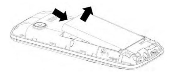
Insert the SIM cards into the appropriate slots under the battery with the contacts facing downwards so that the SIM card contacts touch the built-in SIM contacts inside the phone.
