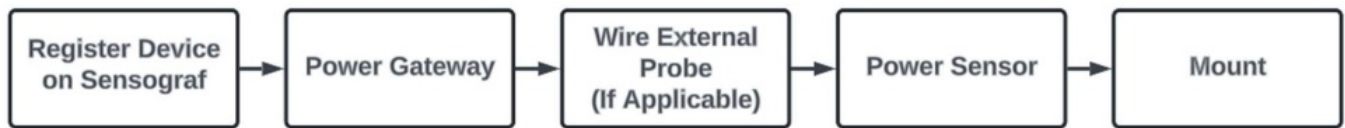
Figure 2: End-to-End Installation of Sensocon-Supplied Sensor, Gateway, & Sensograf Platform
