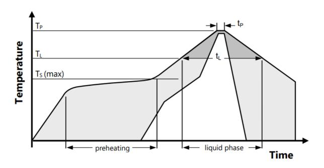
Make sure that maximum temperatures and exposure times are respected. In case the PCB passes through multiple solder cycles (as is the case for e.g. PCBs that are assembled on top and bottom side), it is recommended to assemble the STSxx only in the last solder cycle.
