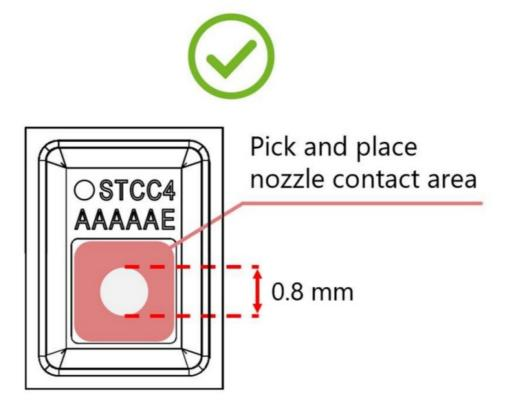
Instruction 4: Pick and place the sensor from within the nozzle contact area, leaving no imprints.
