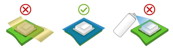
Instruction 6: Do not protect/cover the membrane during a conformal coating process.
