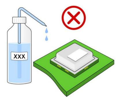
Instruction 5: Do not expose the sensor to strong clean agents before, during or after the soldering process.
