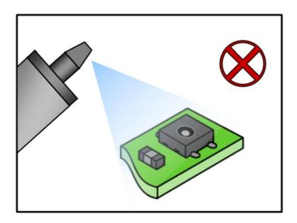
Do not apply spray to unprotected sensors.
