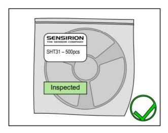
Store sensors in original, unopened ESD bag. Place additional stickers only on the outside of the ESD bag. Once sensors have been removed from the original ESD bag we recommend to store the individual sensors as well as devices with assembled sensors in metal-in antistatic shielded ESD bags. In particular, it is recommended not to use any adhesive or adhesive tapes to reseal the sensor bag after opening. Following ESD Bags can be recommended (no polluting effect on humidity sensor):
