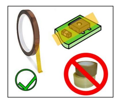
In conjunction with the sensor, use only recommended Kapton® tape Electrical Tape 92 by 3M™. Regarding adhesives and encapsulants, the material in the following tables may be used – according to respective datasheets, applied and fully cured in well ventilated environment (fresh air supply). Materials and brands not listed in the following tables may be harmful and shall be tested carefully before applying.
