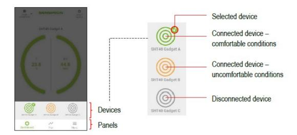
When the gadget logo (concentric circles) is green, it means that the environmental conditions measured by the gadget are deemed comfortable. If a device was connected during the runtime of the application but the connection is subsequently lost, the device logo will appear as grey in the list.
