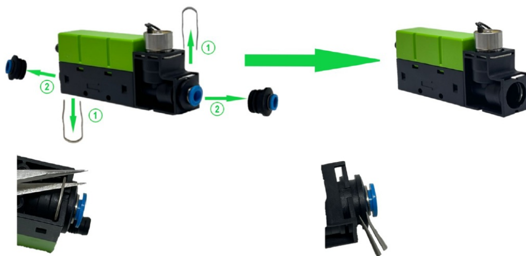
The metal ring for the rear fitting must be accessed from below.
